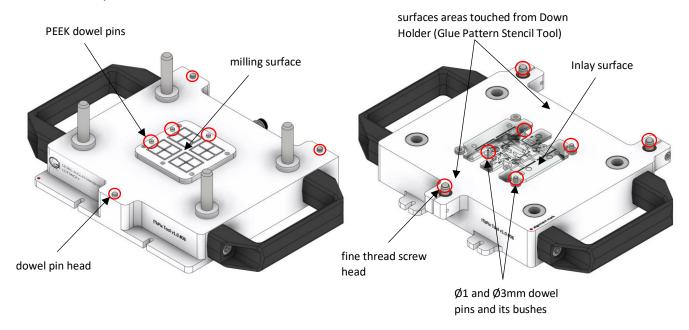
Also, additional parts of the Glue Pattern Stencil Tool, the entire Glue Distributor, entire Glue Pattern Sheet, the Down Holder (Bars) and the surfaces between Down Holder and Glue Pattern Sheet has to be cleaned free of any grime and lint before using and cleaned of glue after using, especially inside of the holes where the glue will collect.
