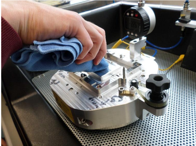
Fig.38 Cleaning baremodule jig contact surface
