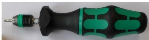
Fig.45 E.g. Torque screwdriver 0.3Nm with corresponding bit SW2.5mm
